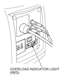
In case of overload operation (refer to page 26) or when trouble occurs for the equipment being used, the output indicator light (green) will go out, the overload indicator light (red) will light continuously, and no power will be put out.
