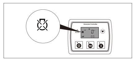
The new generator needs to run-in with low power for about 20 hours, and the load power should be kept within 2000W
