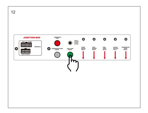
Press and hold the Fuel pump check button with your finger until the fuel is pumped out, and the fuel will come out continuously from the fuel return pipe, which proves that the fuel pipe of the generator is unblocked and installed correctly.
