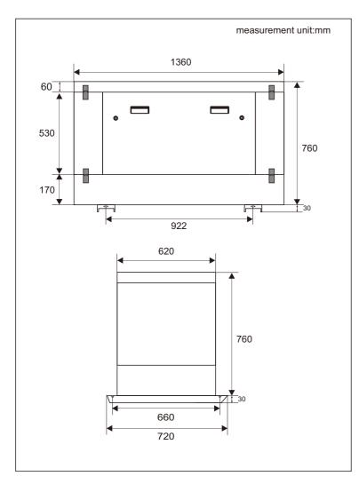
Outside Seawater Exchanger Model: JEC300 CFCS type, 1500rpm.
