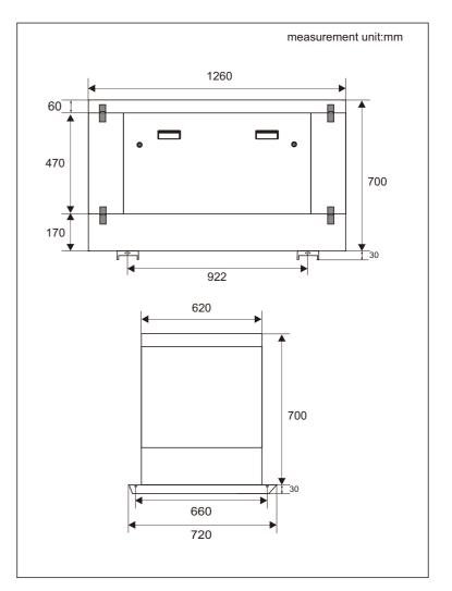
Outside Seawater Exchanger Model: JEC200/250 CFCS type, 1500rpm.
