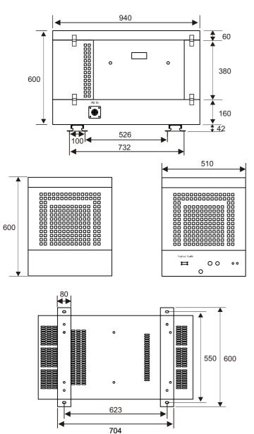
Outside Seawater Exchanger Model: JEC100 CFCS type, 1500rpm.
